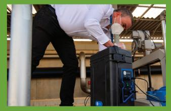
The Aquamonitrix<sup>®</sup> analyser provides an easy way for WWTP operators to accurately monitor nitrite (and nitrate) in real-time, offering the following advantages over conventional sensors:
