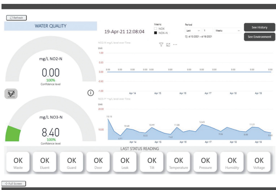
Figure 1: Screenshot of the Datamonitrix report (April 2021) from one of the WWTPs where Aquamonitrix® was deployed in Spain. Datamonitrix is the dedicated data management platform for Aquamonitrix.
